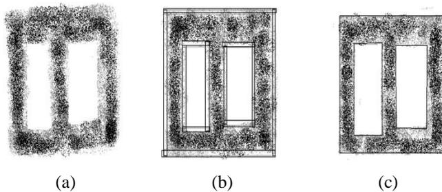
Fig.1. Profile polygons for a large-scale network. (a) Original network topology. (b) Rectangles for smoothing boundaries. (c) Profile polygons.
