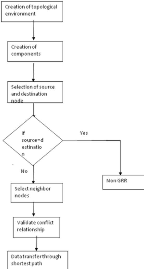
Fig. 3 Data flow diagram of our proposed system.
